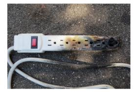
An Air Conditioner and several other devices were plugged into this power strip. The A/C unit was on at the time of the incident.. The increased load from the A/C caused the power strip to overload and catch fire. The A/C unit was also damaged and needed to be replaced.
